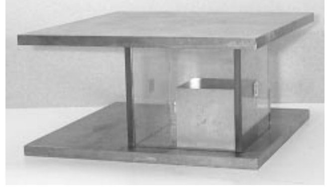
Fig. 6. Photograph of the conducting cube lattice apparatus for measuring quasi-static effective conductivity. The upper and lower plates as well as the cube are brass. The four-sided box is Lexan. For sample #2 shown above, the measured volume fraction was f = 0.1952 \pm 0.0005 , as listed in Table I.
